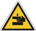
***To prevent serious injury through crushing or amputation, do not work with the equipment without the safety guards installed on the moving parts. Make sure that all the safety guards are correctly reinstalled at the end of the repair or maintenance work of the equipment.***
